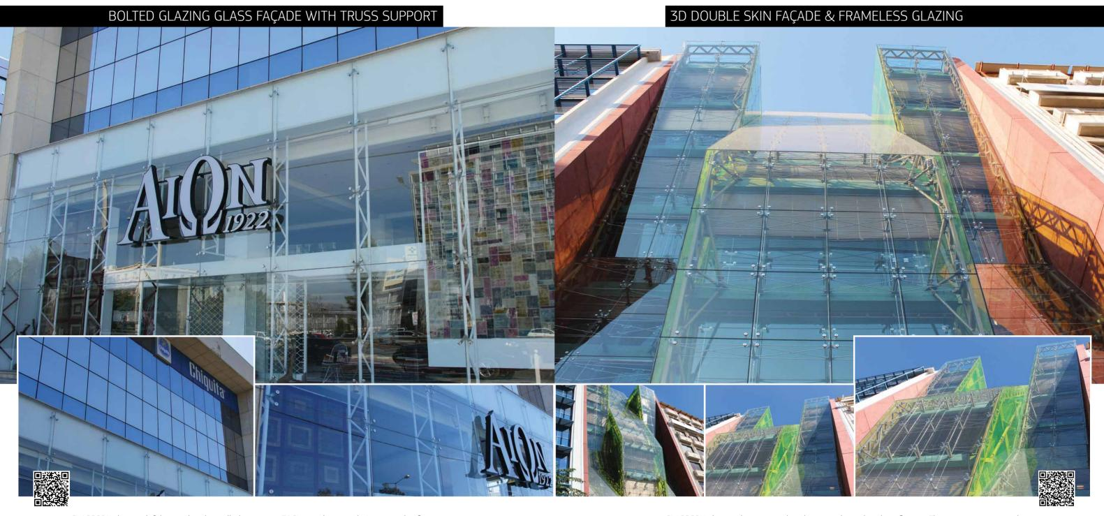
GLASSCON designed, fabricated and installed a spider glass shop front for a large retail shop. The façade is supported by custom made vertical STEEL TRUSSES, co-developed with the project architect. Glass panes are attached to the truss
